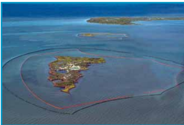
4000 feet of 26" Navy boom surrounding New Harbor Island, Louisiana.
