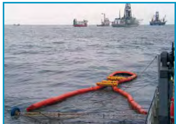
SUPSALV's Vessel of Opportunity Skimming System (VOSS) oil containment booms deployed.
